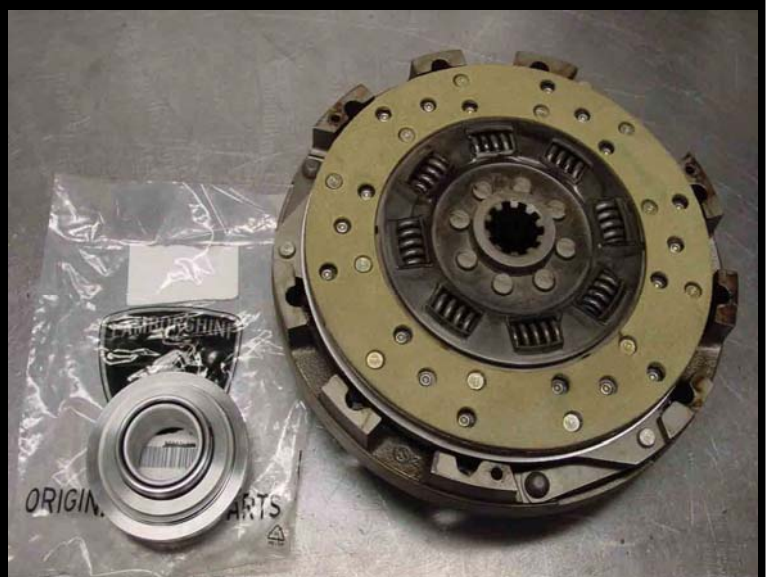
A kevlar clutch for a newer model Diablo
