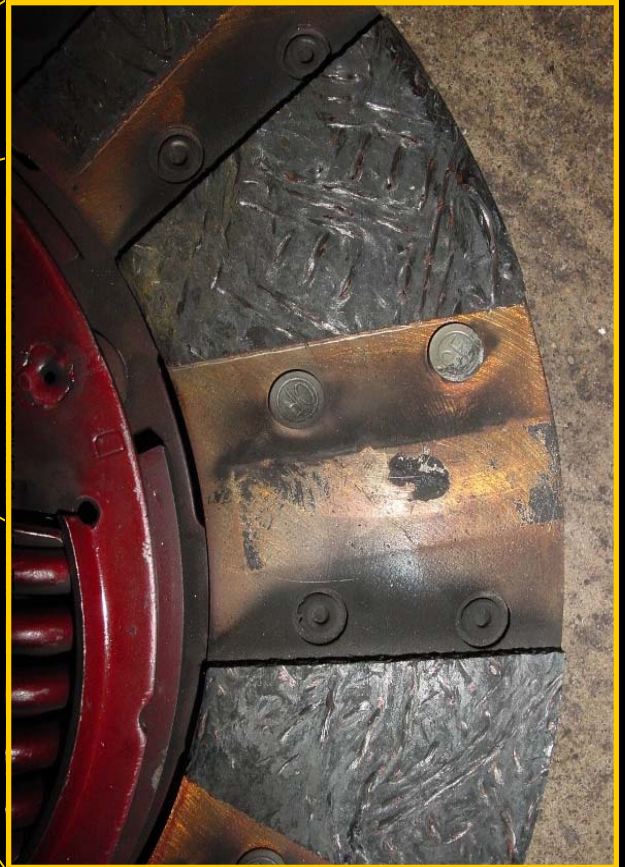
A failed carbon fiber clutch disk belonging to another Midwest Diablo owner, notice the missing section of clutch lining
